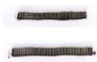
Weight per unit of length for chips generated by the inner edge (In-house evaluation)
